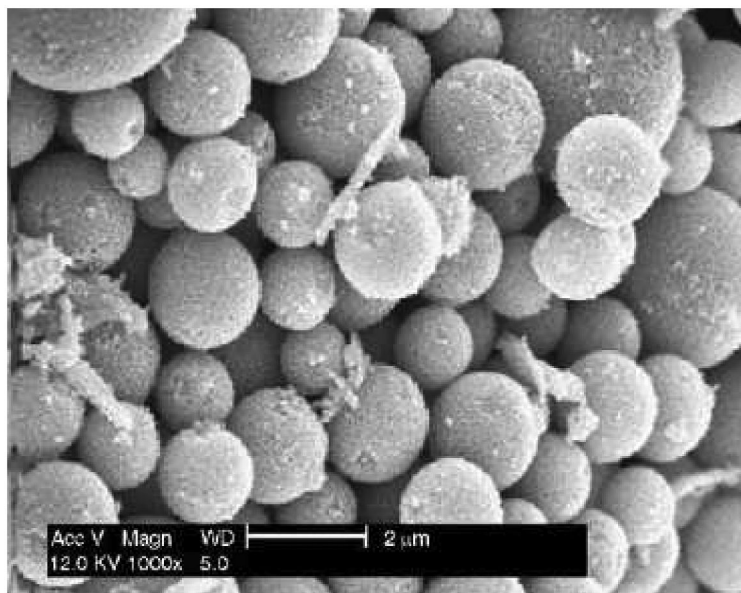
Figure 1. SEM image of the \text{WO}_3 microspheres, reproduced from (18).
